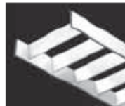
S79 Parabolic Baffle 1-1/4" high blade, 2.4" o.c., semi-specular low-brightness Pearlescent Aluminum baffle. Continuous and unbroken, no visible joints.
